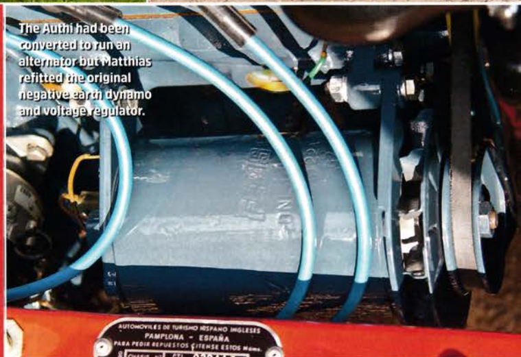
Wiring up the FEMSA voltage regulator was time-consuming, with no diagrams for guidance.
